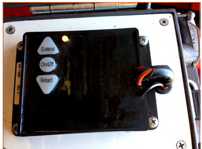
Manual Controls for the 4th cylinder on the hitch assembly.
