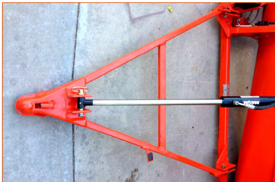
Hitch assembly connected to the cylinder #4 and ready to connect to the tow vehicle.
